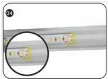
04 Note that the cut marks are the locations of electrical contacts. Ensure these are isolated with the adhesive tape the avoid short circuits
